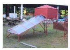
Figure 9. Setting up the metal frame with stainless steel sheet and polyethylene plastic cover for the solar dryer for coconut male flowers
