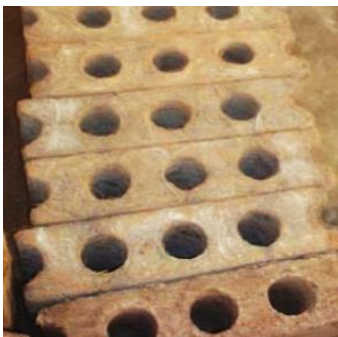
Coir-reinforced Cement Hollow Blocks
