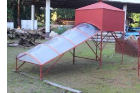
Figure 9. Setting up the metal frame with stainless steel sheet and polyethylene plastic cover for the solar dryer for coconut male flowers
