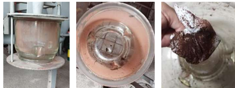
Figure 14. Tannin powder produced one (1) gram at one (1) hour operational testing
