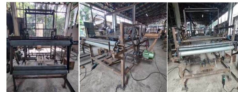
Figure 11. Installation of the metal frame, steel rollers, and steel braces for the mechanized coir looming machine
