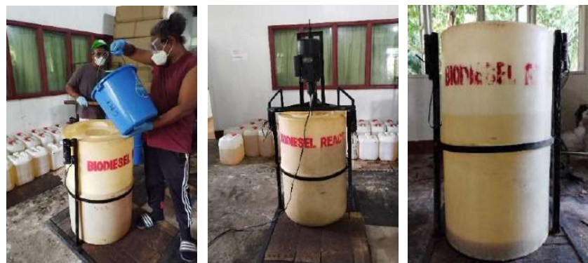
Figure 25. Actual operation of the trans-esterification process of crude coconut oil
