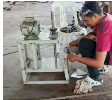
Figure 12. Fabrication of body frame of pneumatic buko trimmer
