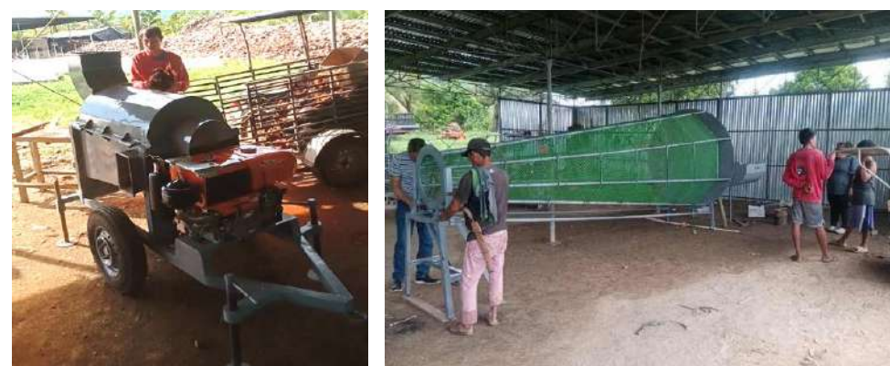
Figure 21. Training on operation and maintenance of Decorticating Machine and Rotary Horizontal Sieving Machine
