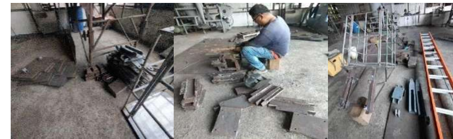
Figure 10. Setting up the metal frame for the harvester platform and preparing metal components for the modified ladder for near-crown coconut operations
