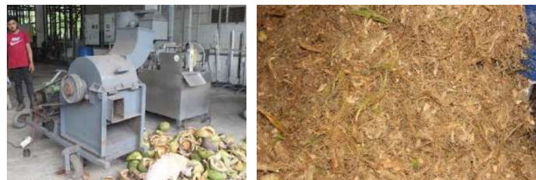
Figure 16. Testing of biomass shredder using 5hp induction motor
