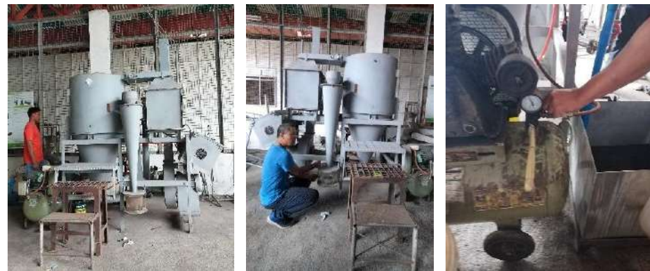
Figure 13. Functional testing of Spray Dryer Machine using tannin extract sample
