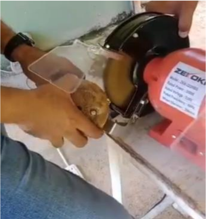
Actual prototype of the Coconut Shell Smoothing Machine
