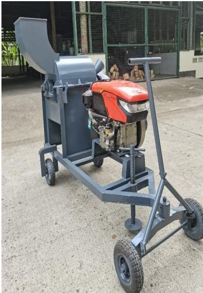
Actual prototype of Biomass Shredder with Wood Chipper
