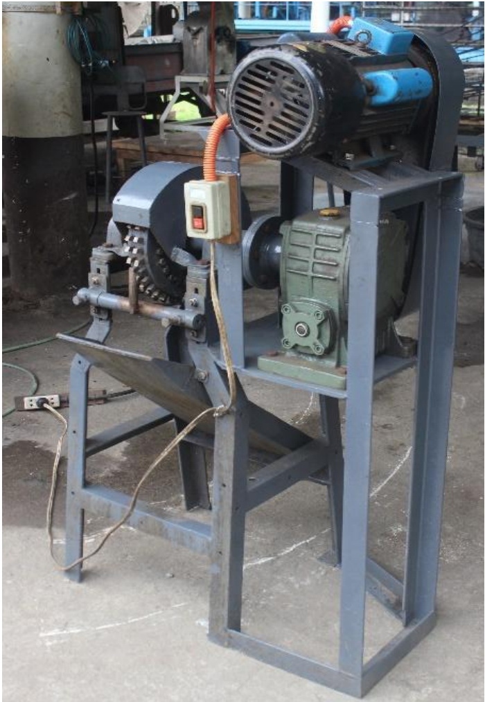
Actual prototype of the Coconut De-sheller
