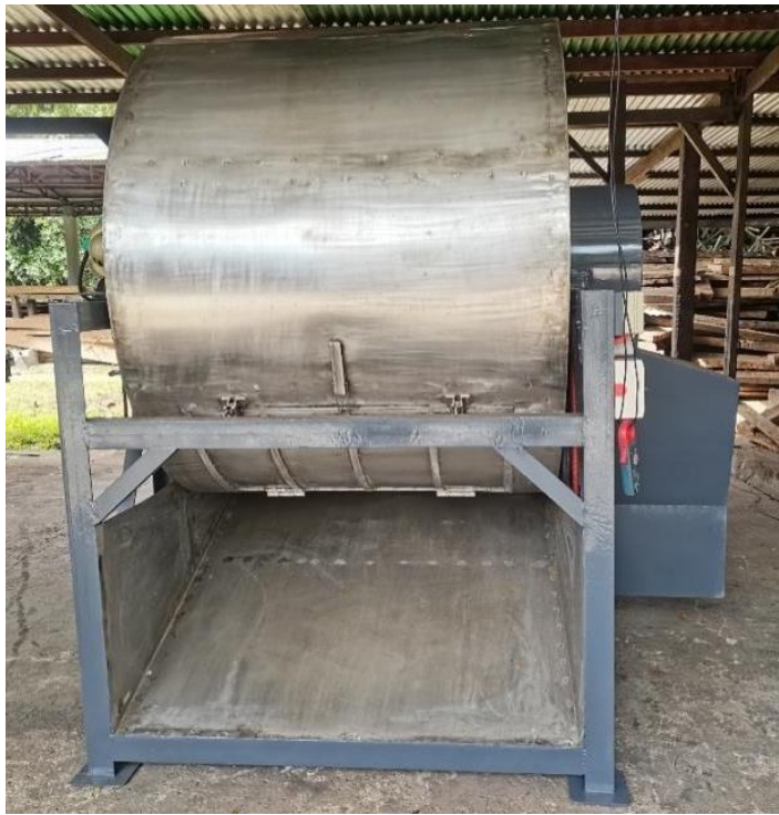
Actual prototype of Rotary Composter
