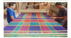
Coir blinds are for decorative purposes. Bleached and dyed coir twines are weaved manually in a looming machine. The weaving will take one meter per day to make. The coir blind will take a week to produce (including treatment coir, and coir twining).
