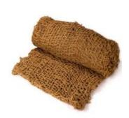
Coir geonets are made from untreated coir, twined and weaved. The production of this geonets will take ten meters per day. The geonet's main application is to prevent landslides in landslideprone areas. Geonets are eco-friendly and will decompose over time.
